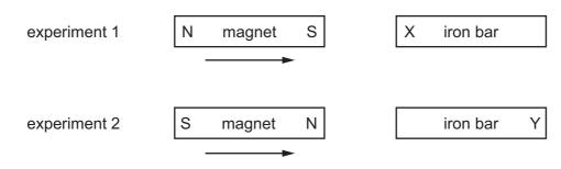
Which magnetic pole is induced at X and at Y?
