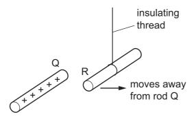
When the positively charged rod Q is brought close to rod R, rod R moves away from rod Q.
